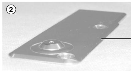
3. Loosen the set screw (upper side) of pressure foot and unscrew the set screw (lower side).
