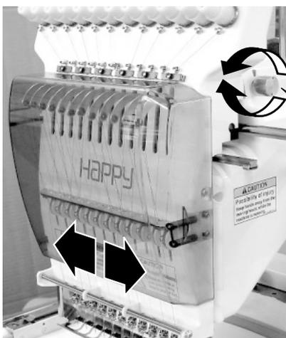
Turn the needle bar selection knob to the marked area with hand.
