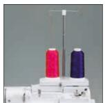
Detachable 2-pin spool stand for large thread cones. Perfect for quick thread changes or twin-needle sewing.
